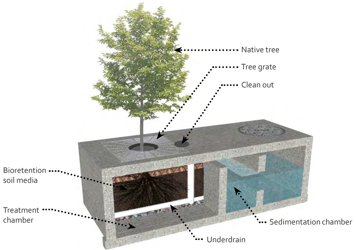
FIGURE 3.6. TREE BOX FILTER
