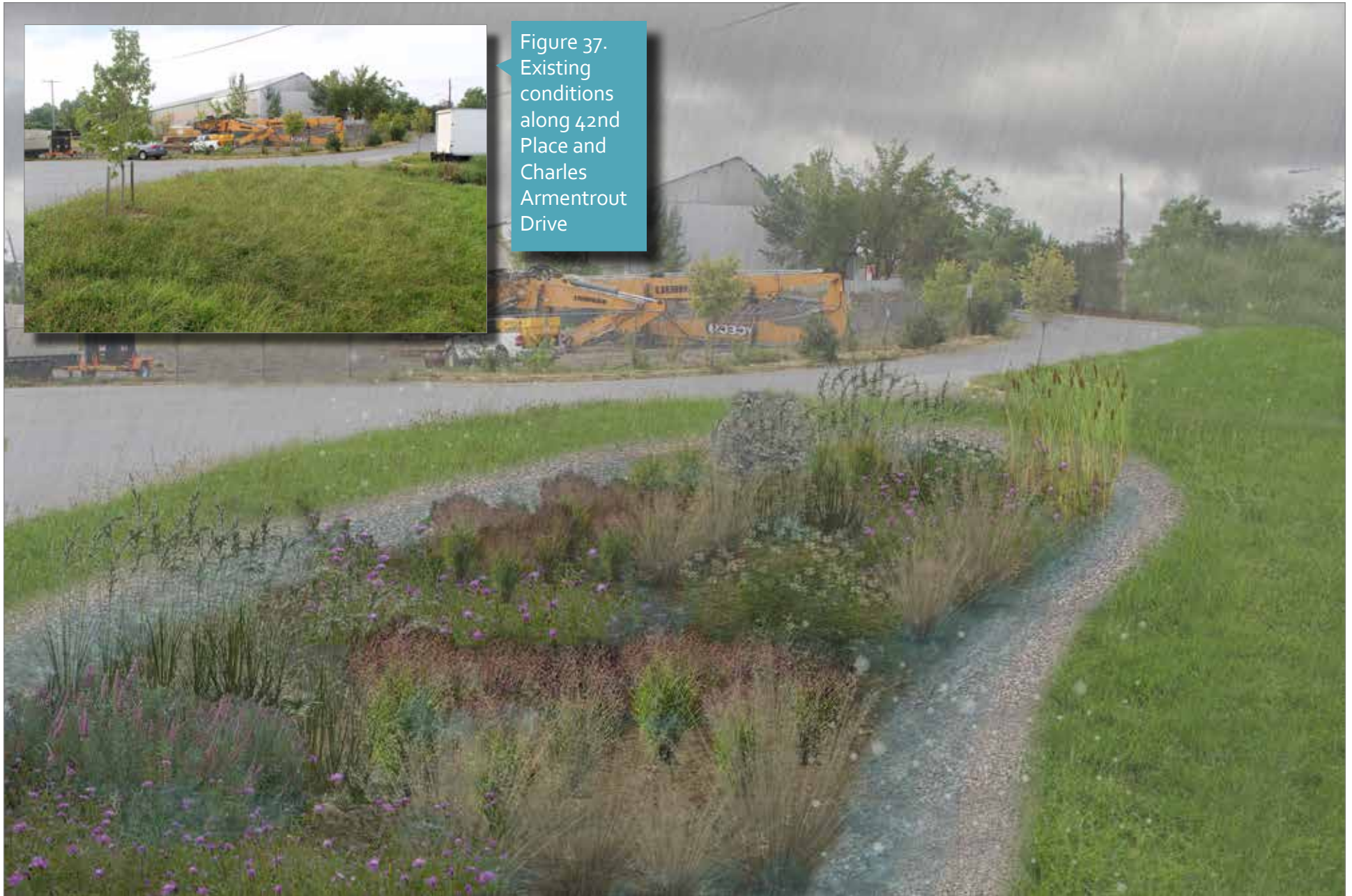
Figure 38. Rendered overlay of submerged gravel wetland project along 42nd Place and Charles Armentrout Drive
