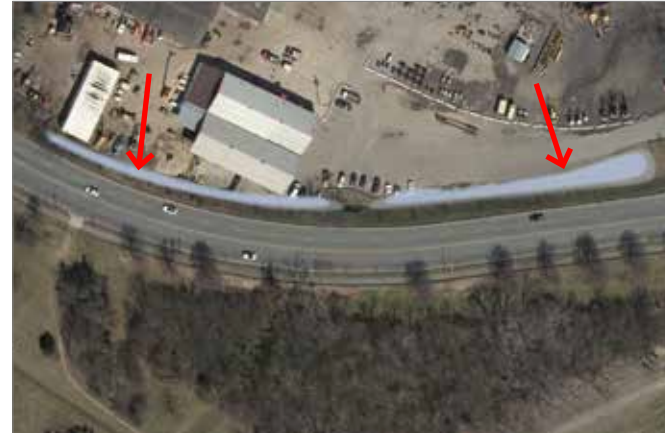
Figure 34. Conceptual overlay of bioswale along Charles Armentrout Drive
